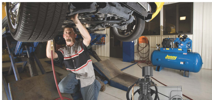
Air leaks cost shops hundreds of dollars a year in energy costs and compressor wear. Find most leaks after hours by just listening for them when the shop is quiet.
