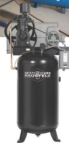
Piston compressors (here, with an exposed piston), are the most common systems in the U.S.
