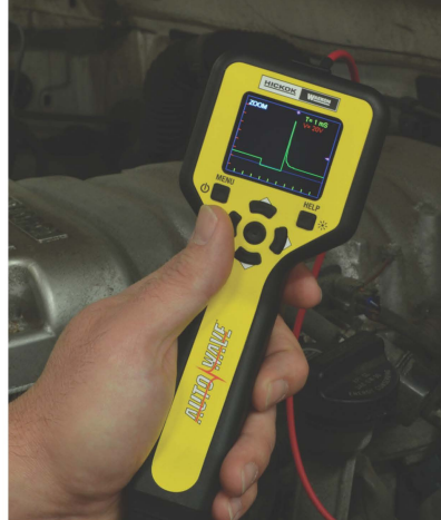
A simple wave form viewer like this one from Hickok can quickly check the pattern of a single component.
