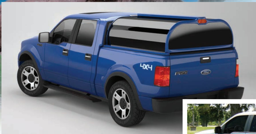
Right: Several truck caps, like this fiberglass one from ATC, provide users with such built-in features as LED brake lights, heavy-duty rear door and oversized windows.
