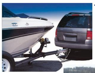
Hitch makers are challenged with the critical task of designing vehicle-specific hitches with greater tongue weight that flex under load. This, and the ever-changing nature of vehicle body designs, has led to a trend toward more vehicle-specific, custom fit hitches versus the old universal "multi-fit" hitch. Photo at left from Cequent.
